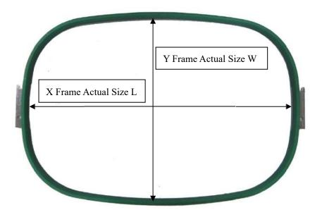
"X direction frame size" and "Y direction frame size" should be set according to the actual size of different frames. Note: this parameter need be set according to the actual embroidery range of the frame, for the apparel frame is usually not square.
